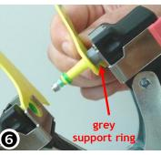
Pliers are supplied with a grey support ring on the metal guide pin in order to support the male part of the tag on insertion. If the support ring becomes detached - clip back into place.
